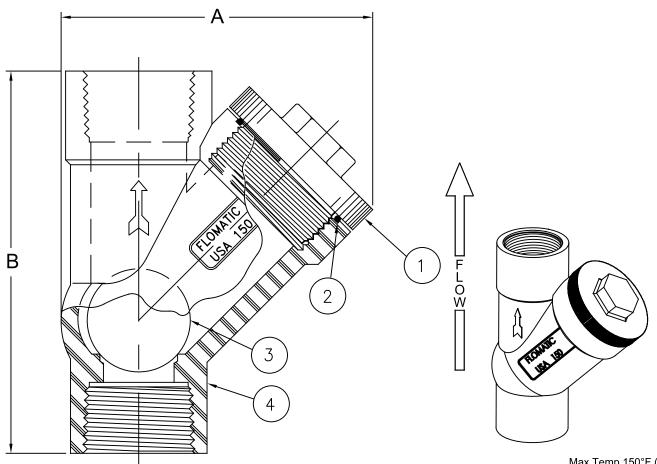
Max Temp 150°F (65°C) Max Inlet Pressure 100 psi (7 bar)
