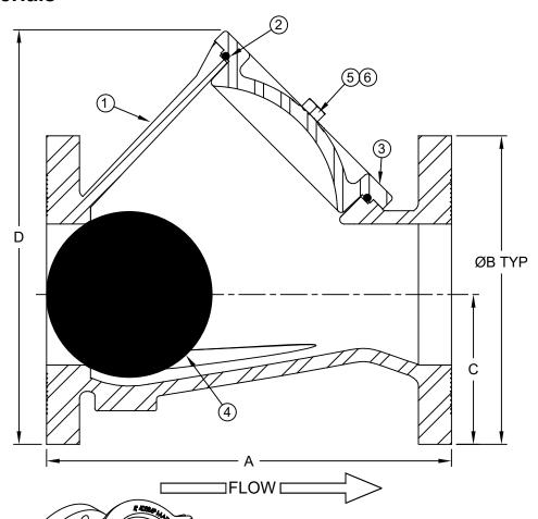
Max Temp 180°F (82°C) Max Inlet Pressure 150 psi (10 bar)
