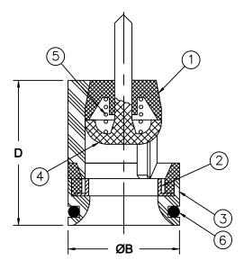
Max Temp 180°F (82°C) Max Inlet Pressure 150 psi (10 bar)
