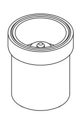
Max Temp 180°F (82°C) Max Inlet Pressure 150 psi (10 bar)
