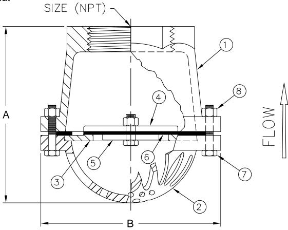
Max Temp 80°F (27°C) Max Pressure 20psi (1.4bar)
