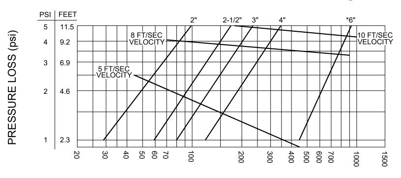
FLOW RATE (gpm) verified by independent lab
