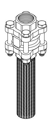
Open Area: 25-30% Max Temp 400°F (200°C) Max Pressure 300psi (21bar)
