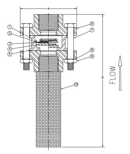
Open Area: 25-30% Max Temp 400°F (200°C) Max Pressure 300psi (21bar)
