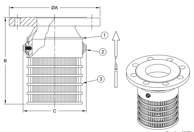
Open Area: 35-50% Max Temp 180°F (82°C) Max Pressure 250psi (18bar)
