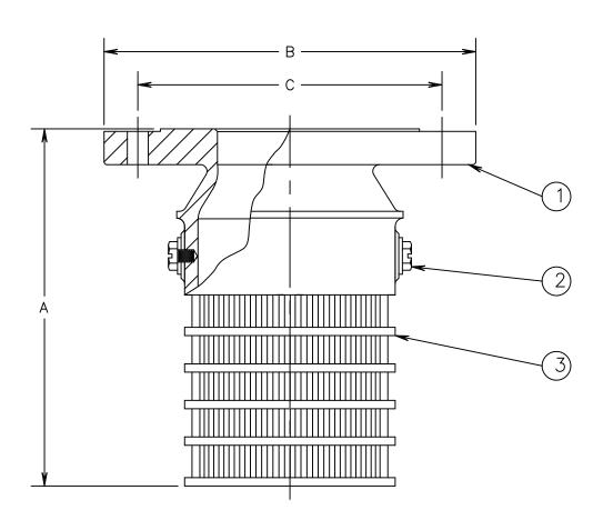
Open Area: 35-50% Max Temp 180°F (82°C) Max Pressure 250psi (18bar)
