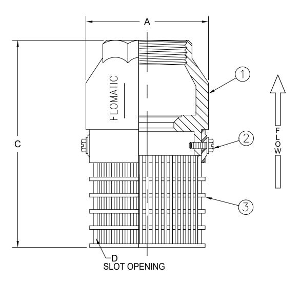
Open Area: 35-50% Max Temp 180°F (82°C) Max Pressure 250psi (18bar)
