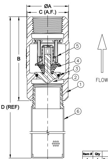
25-30% Screen Material Open Area Max Temp 180°F (82°C) Max Pressure 400psi (28bar)
