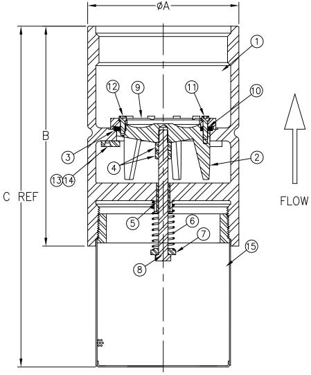
Max Temp 400°F (200°C) Max Pressure 400psi (28bar)
