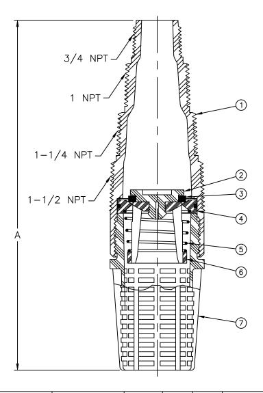
Open Area: 30-40% Max Temp 140°F (60°C) Max Pressure 150psi (10bar)
