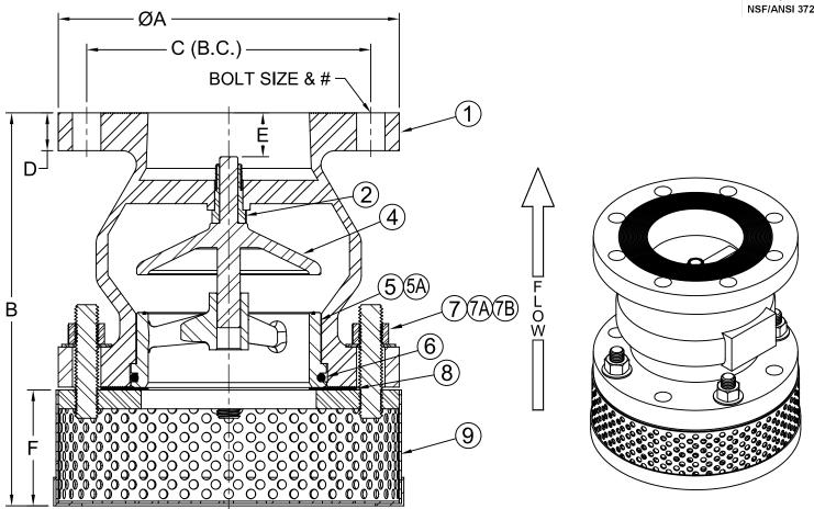
Max Temp 200°F (93°C) Max Inlet Pressure @ 100° F (38°C) 275 psi (19bar)
