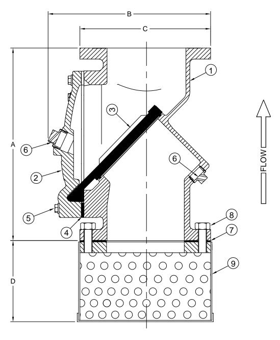
Open Area: 50-60% Max Temp 140°F (60°C) Max Pressure 250psi (18bar)
