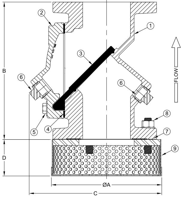
Open Area: 50-60% Max Temp 140°F (60°C) Max Pressure 250psi (18bar)
