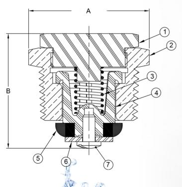
PRESSURE MAX: **400 PSI** TEMP MAX: **180°F** SIZE: **1"**Connection: 1" NPT Male Connection
