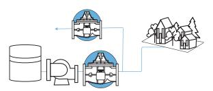
Protect against surges in a pump station resulting from power failure when the pump discharge valve is a slow opening and slow closing pump control valve
