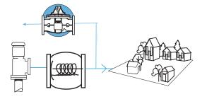
Protect against surges in a deep well pump station which occur during start up, shut down, and power failure when the pump discharge valve is a conventional check valve, such as swing, silent, or double door types.
