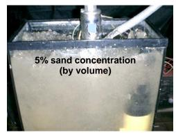
Test tank in above left picture shows a submersible test pump with two circulating pumps. Test tank on the right shows 5% sand concentration by volume. The two circulating pumps on each side of the test pump are keeping the sand/water concentration in suspension during valve cycling test. A typical stem type check valve under the same test condition will not be able to handle even 0.25 % or a ½ % sand solution.
