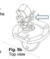
**Function:** The limit switch when probably adjusted will give an electric "closed" and/or "open" circuit when valve is open and/or in closed position.
