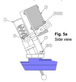
The limit switch option (Model 745LS) is factory installed or field installed (see Fig 5a & 5b) on the valve access cover and is used in conjunction with the Position Indicator (PI). A standard limit switch (Honeywell Model LSH1A or Equal) is mounted on an epoxy coated steel bracket for easy wiring, field adjustments and servicing. The limit switch is SCADA (Supervisory Control and Data Acquisition) compatible for applications requiring open/close indication.
