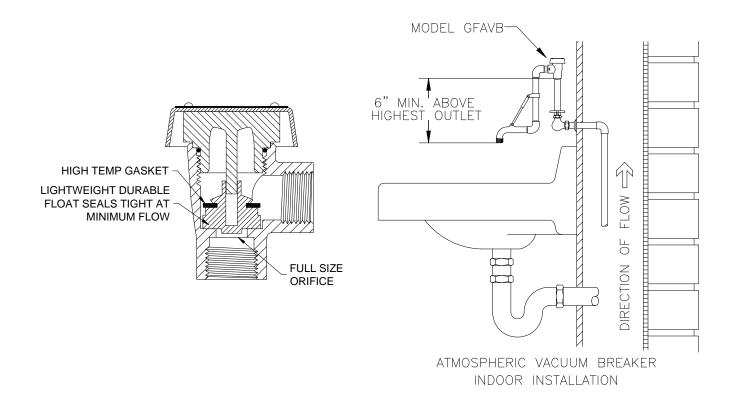
CAUTION: This device should never be used in installations that are under continuous pressure. Therefore, never place a shut-off or check valve downstream of GFAVB's.
