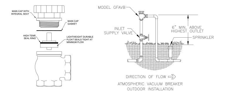
CAUTION: This device should never be used in installations that are under continuous pressure. Therefore, never place a shut-off or check valve downstream of GFAVB's.
