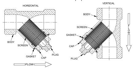
Make sure the pipe is aligned so it is straight and threads into the Flomatic® Y-Strainer. Make sure the cap is not offset or at angle when being installed. The plug may be removed for a Blow-Down Valve to be installed.
