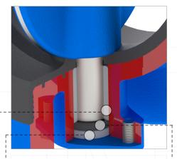
Thrust Bearing: Nylon Shaft Support.
