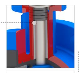
**Upper Shaft Bearing: 304 Stainless** Steel. Teflon Coated.
